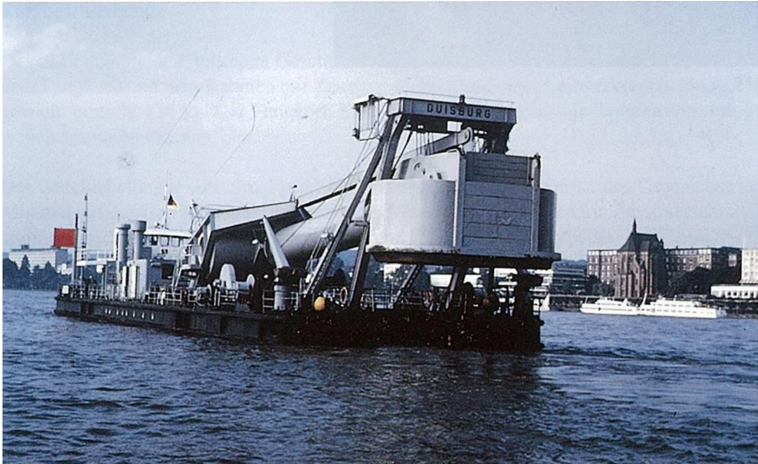
Special boat for bottom sediment sampling
