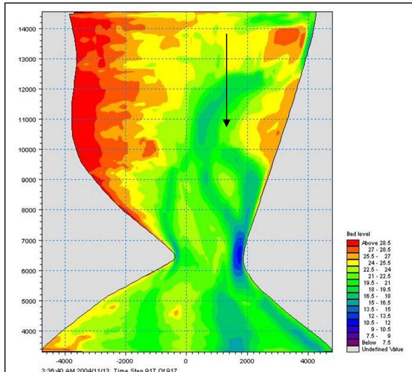
**Figure 4-5** Simulated bed level (masl) at end of flood (flood peak 25000 m<sup>3</sup>/s, hydrograph duration 2.5 months)
