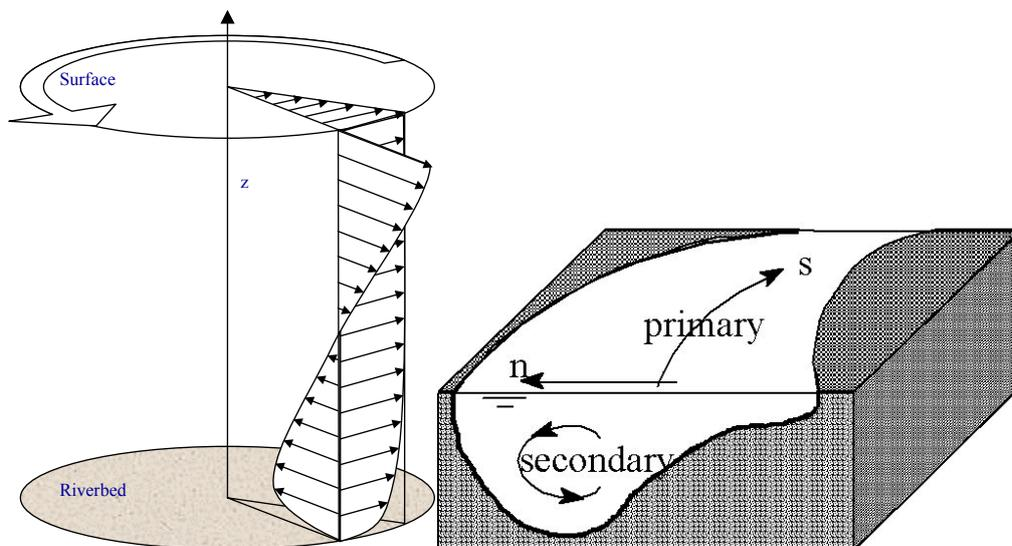
**Figure 4-1 Profile functions in pseudo 3D model (DHI, 2003)**
