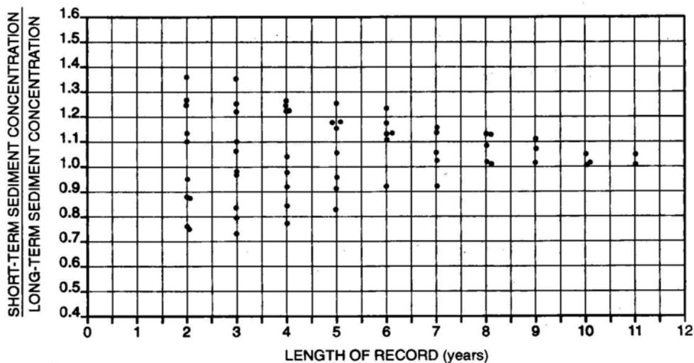
**Figure 3-5 Short-term effective sediment concentration compared with long-term concentration on the Orange River (Rooseboom, 1992)**
