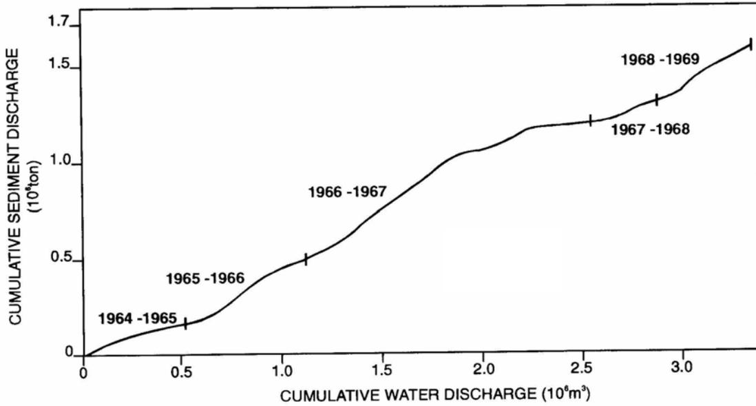
**Figure 3-3** Cumulative sediment load versus discharge relationship on the Orange River, South Africa (Rooseboom, 1992)
