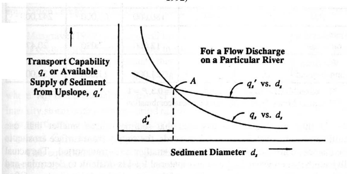
Figure 3-2 Concept of controlling sediment transport rates (Shen, 1971)
