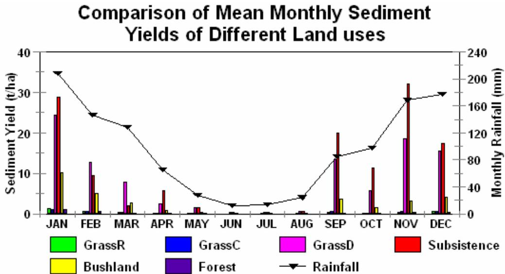
**Figure 3-7 Comparison of sediment yields simulated under different land uses in Subcatchment 6. Under grasslands, R designates rehabilitated (i.e. well managed) conditions, C current and D degraded (overgrazed) conditions (Dlamini and Schulze, 2002)**
