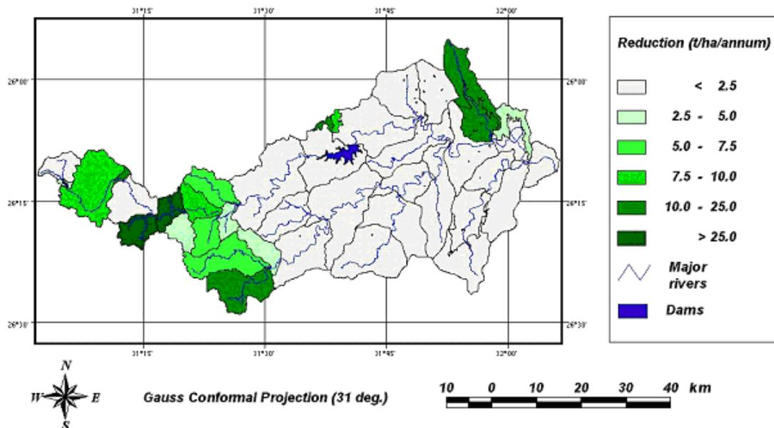
**Figure 3-8** Absolute (t/ha) differences between simulated mean annual sediment yields under rehabilitated vs degraded conditions (Dlamini and Schulze, 2002)
