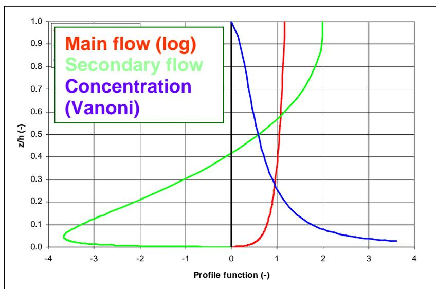
**Figure 4-2 Vertical flow and concentration distribution (DHI, 2003)**
