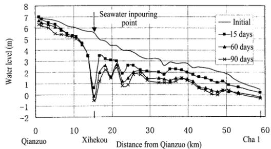
Fig.3.5 Changes in longitudinal profile of the Yellow River mouth after diversion of seawater
