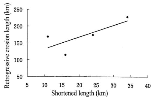
Fig.3.3 Relation between retrogressive erosion length and shortened length (Zhang, et al. 2005)
