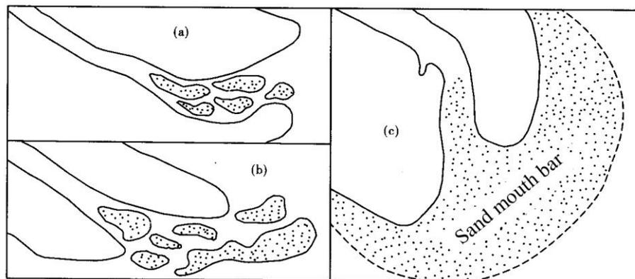
Fig.2.6 Plane configuration of the mouth bar
