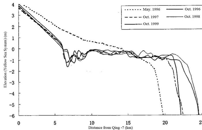
Fig.2.7(b) Longitudinal profile of the mouth bar after Qing-8 forking
