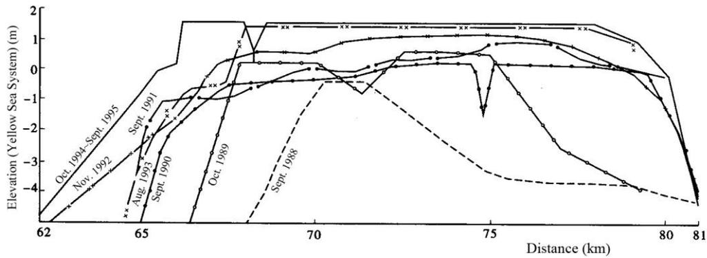
Fig.2.8 Changes of the mouth bar in Cross-section
