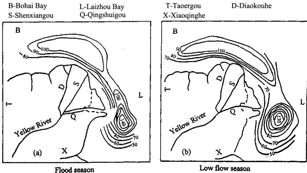
Fig. 2.3 Sea current velocity contour near the river mouth (Unit: cm/s)
