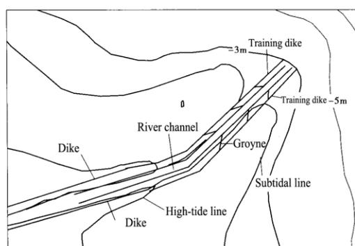
Fig.3.4 Plan view of the double training dikes in the Yellow River mouth
