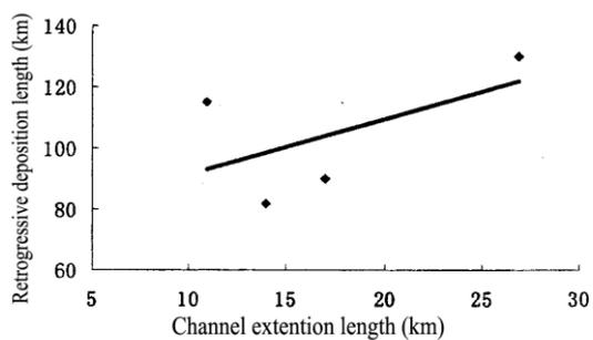
Fig.3.2 Relation between channel extension length and retrogressive deposition length (Zhang, et al. 2005)
