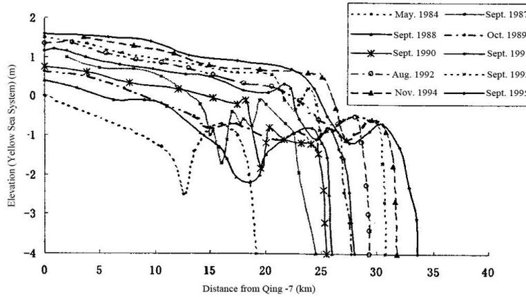
Fig.2.7(a) Longitudinal profile of the mouth bar before Qing-8 forking
